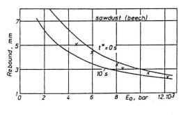
Fig. 9. The rebound of the pressed sawdust.
