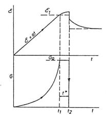
Fig. 2. Creep and rebound of the compressed material.
