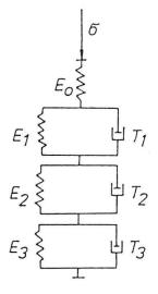
Fig. 1. The extended three-element model.
